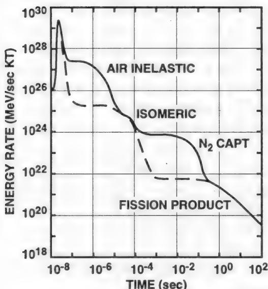
**Figure 8.1.** Idealized Time Dependence of the Gamma-Ray Output from a Large Yield Explosion, Normalized to 1 KT.
